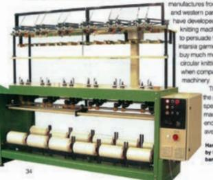
Harry Lucas' RR3-Z-108 is one of four single jersey machines developed by the company for producing corals, shoelaces, various trimmings, bandages, isolation components, artificial veins, and effect yarns.
